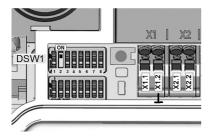
The use of the domestic connection monitoring function with RS485 meters must be selected using a DIP switch setting and does not come into effect until the Wallbox has been restarted. If no meter **5** is found when the ModBus function has been enabled, the charging current is reduced to 10 A.
