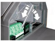
2. Press the screwdriver into the supply terminal.
