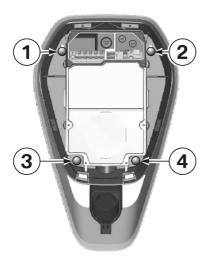
1. After inserting the cable, attach the Wallbox to the two top wafer-head screws 1 and 2.
