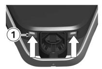
Press the two interlocks 1 for the housing cover on the underside of the Wallbox upwards.
