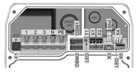
Mains connection outer conductor 1
