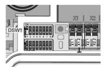
The use of the enable input must be activated by a DIP switch setting.
