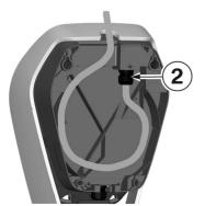
Route the supply cable in a loop to the cable gland 2. Comply with the maximum bending radii of the cable.
